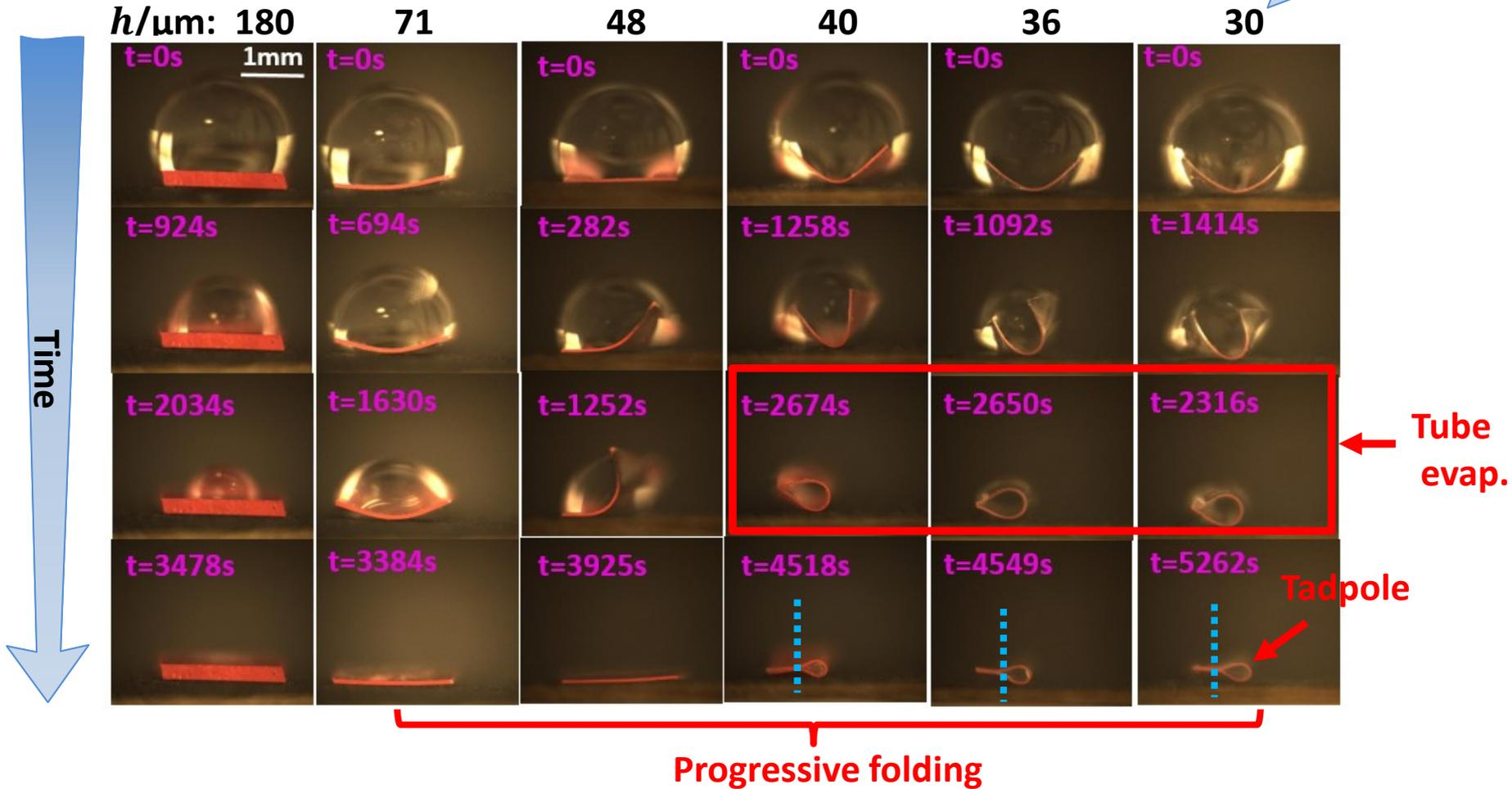
Folding process of flexible membranes (side view)
